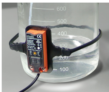
A sensor can be set to detect low fluid level in your mobile phase container.
